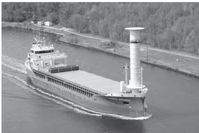
M/v Annika Braren z rotorem. Fot. WASP photogallery https://northsearegion.eu/wasp/photo-gallery/
